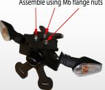
6.Attach turn signals to bracket B using bolts G and crush tubes F.
